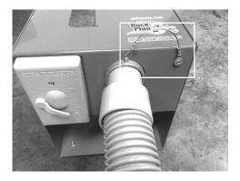
Your Big Blue Blower will accept standard 1-1/2'' hose fittings on the inside of the blower opening. In most situations the friction fit should be sufficient to keep the hose in place. However additional hold can be achieved by using the attached retainer pin. To use the pin you will have to drill a hole into the hose fitting you will be using.
